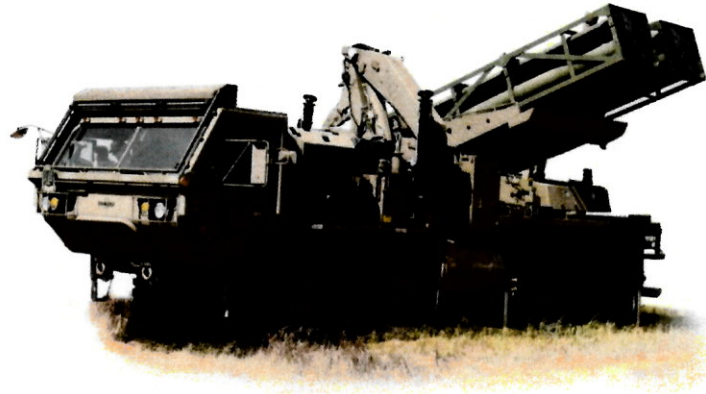
Figure 6: PULSTM™ mounted on an 8X8 platform (IDF)
