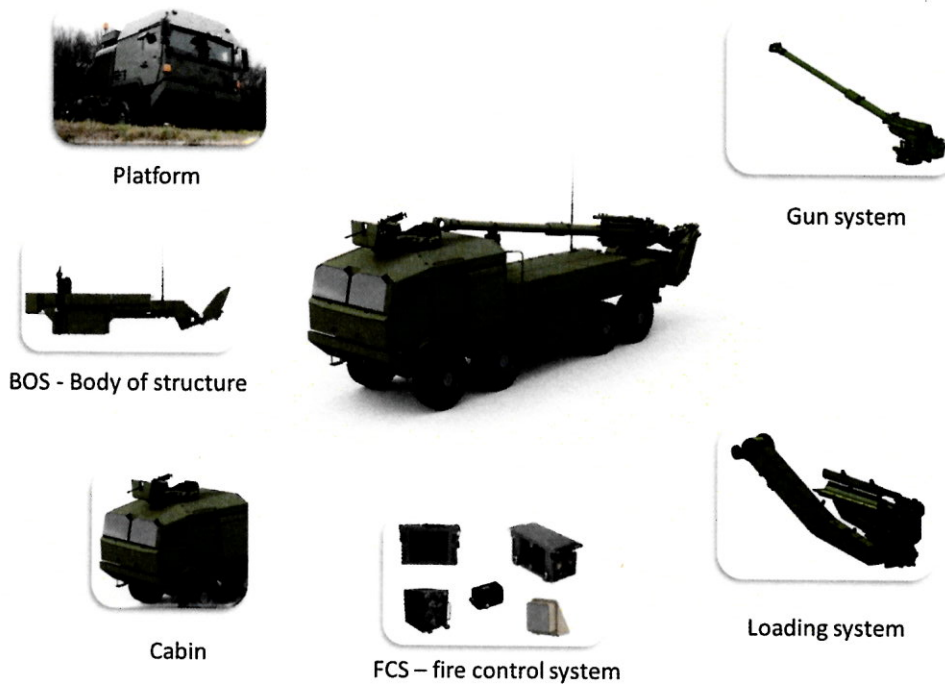
Figure 4: ATMOS - Modular Design (Illustration)
