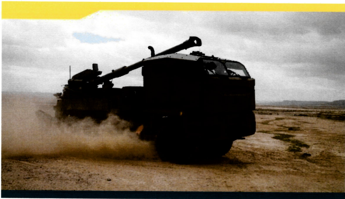
Figure 1: On-the-Move – ATMOS on MAN TGS truck (Illustration)
